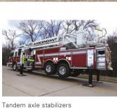
1,000' of 5" or split load 700' of 5" & 600' of 3" hose Hosebed Capacities 1,000' of 5" hose Ladder Minimum of 115' Minimum of 115' Complement Ladder Warranty 20-yr structural 20-yr structural
